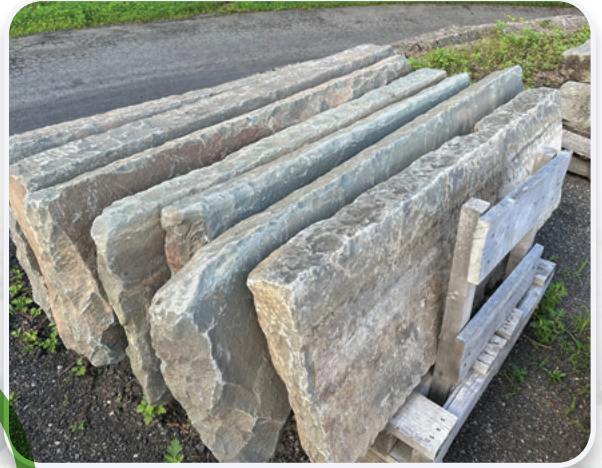
Reclaimed Bluestone Curbing
